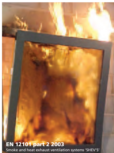
ABOVE Picture of EN12101-2 AOV in a fire test (Annex G)
